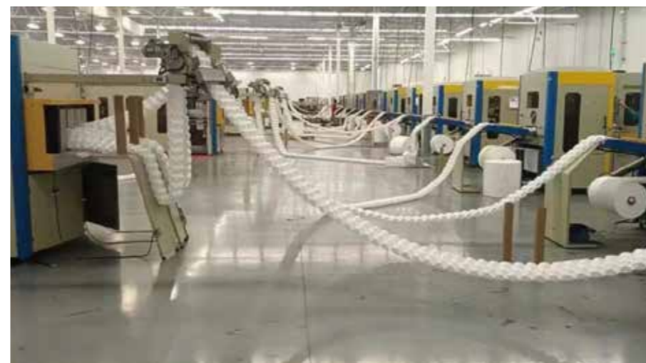
袋装弹簧生产线车间实景 Pocket spring production line
