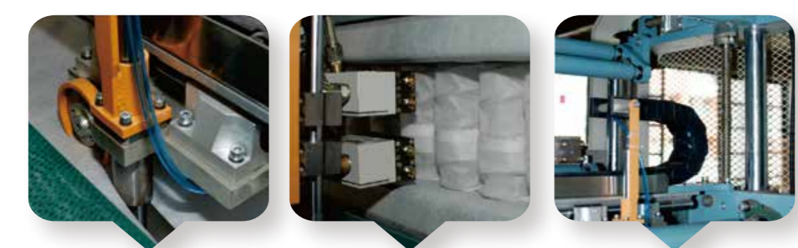
电动上下布裁切装置 Electronic control cutting device for the top&bottom fabric 可独立开关的喷胶头 Independent hot melt jets 电动粘胶平台升降装置 Electronic control assembling platform for pocket spring units
